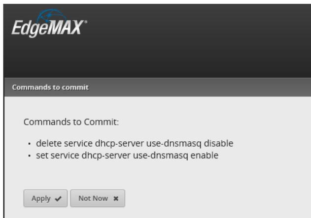
**Figure 32 – Example of Multiple Config Tree Commands**
